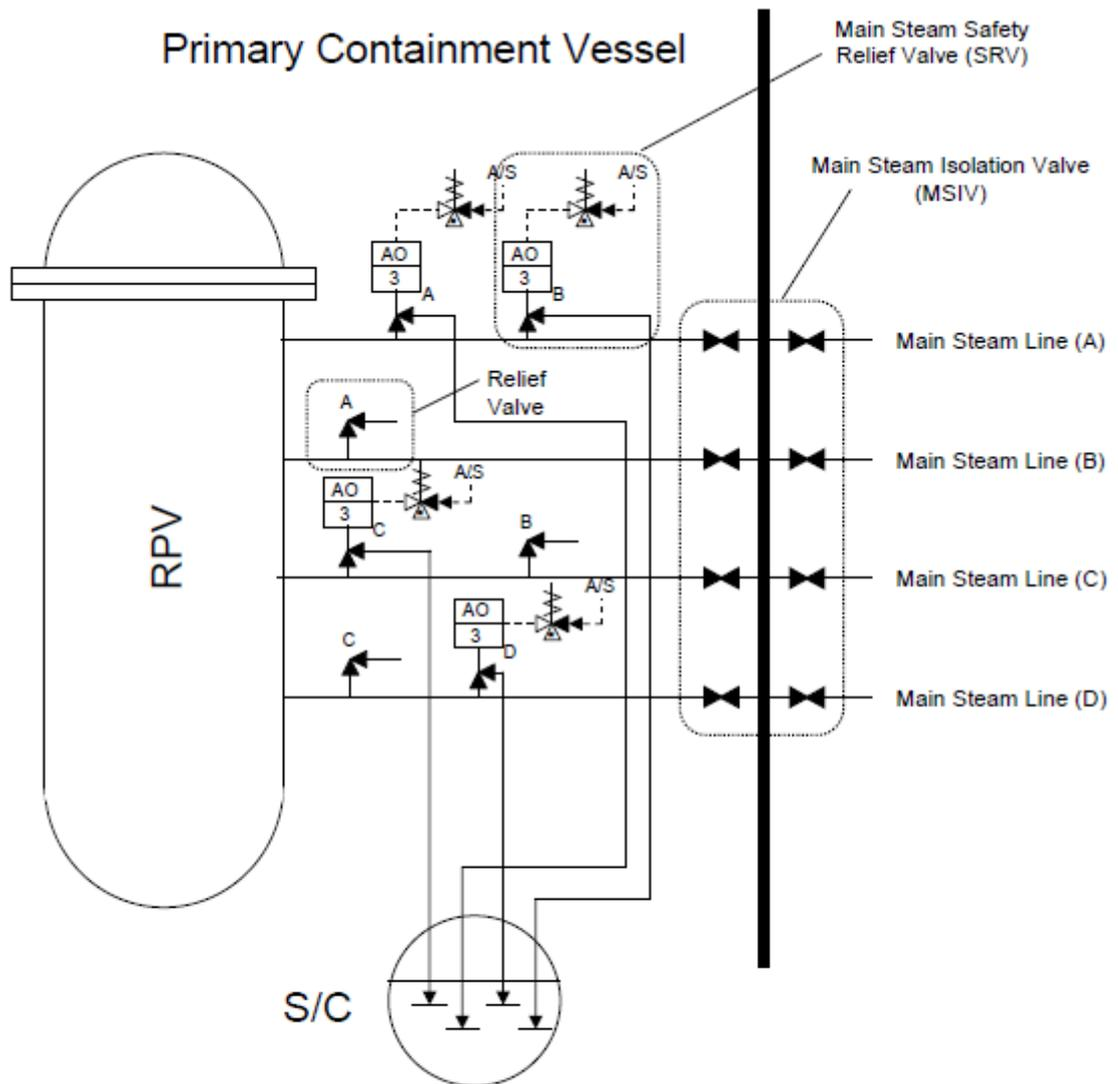
\*1: The main steam safety relief valves (4 valves) are AO valves, and open drive air is supplied by the energized solenoid valves of air supply lines. During power loss, solenoid valves become deenergized and main steam relief valves are in a closed condition.
