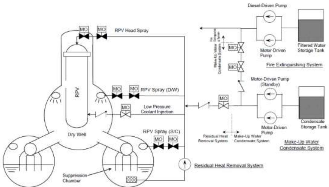
Figure IV-2-11 Overview of the Alternative Water Injection Facility for Units 2 and 3
