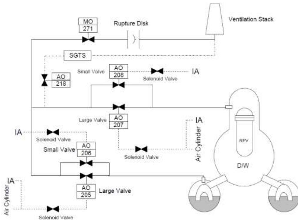
Figure IV-2-14 Overview of PCV Venting Facility (Units 2 and 3)
