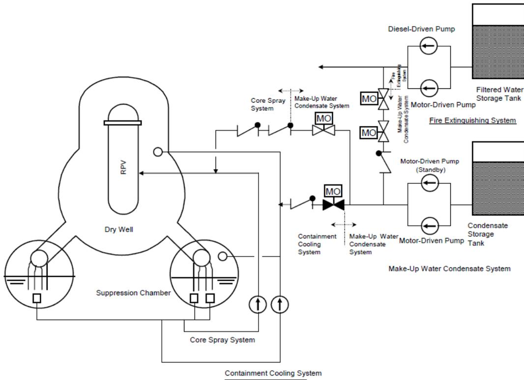
Figure IV-2-10 Overview of the Alternate Water Injection Facility for Unit 1
