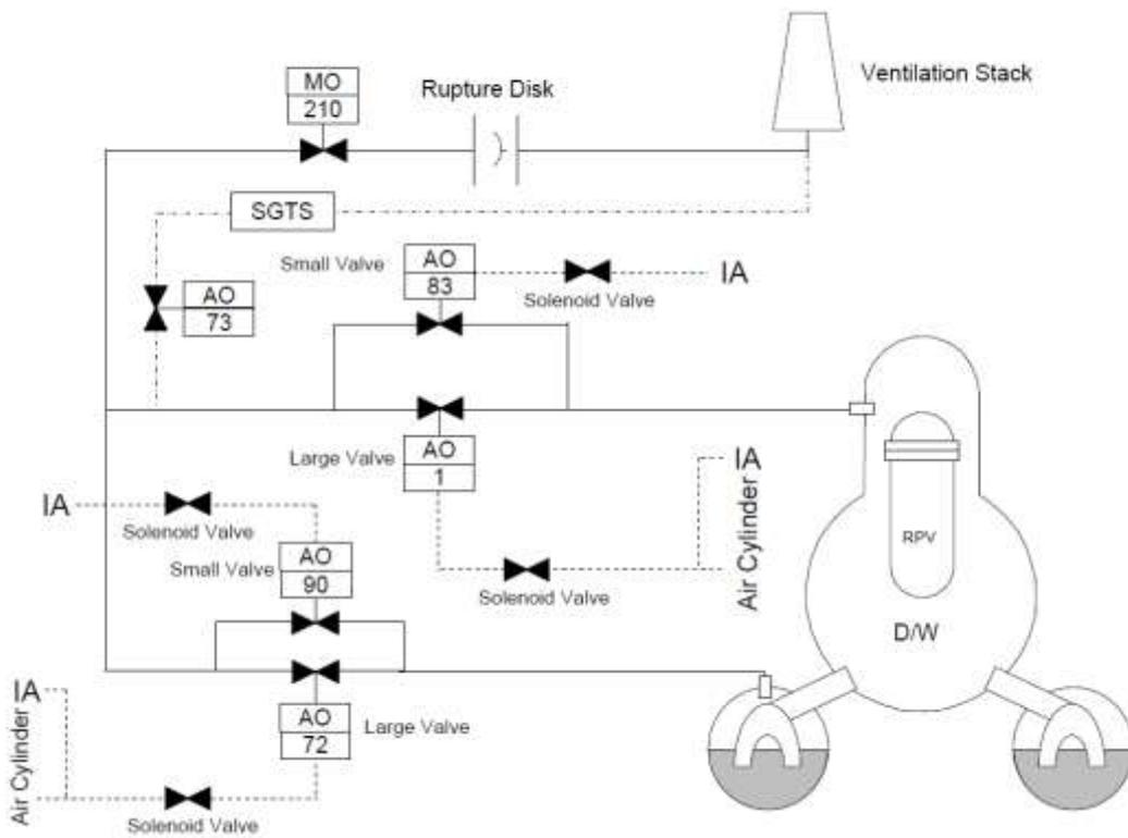
Figure IV-2-13 Overview of PCV Venting Facility (Unit 1)
