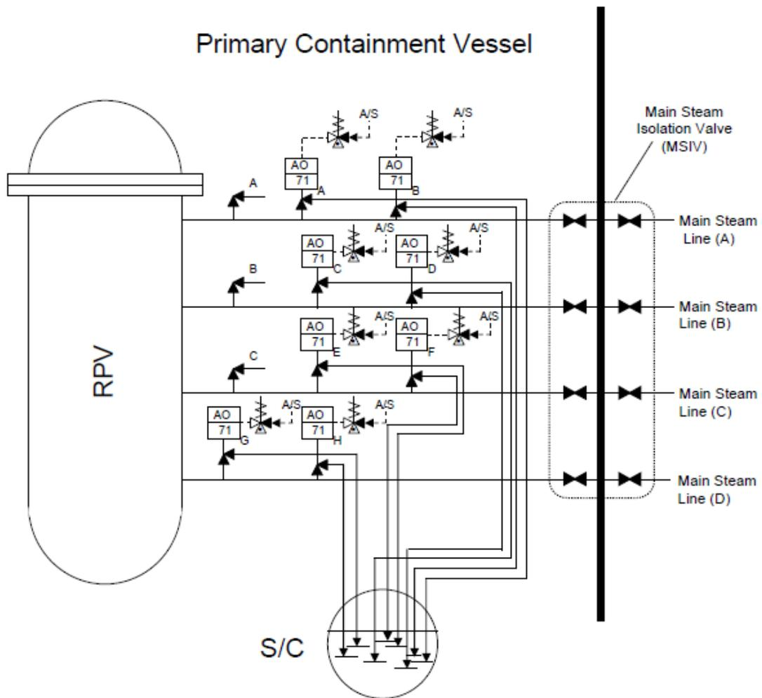
\*1: Main steam safety relief valves (8 valves) are AO valves, and open drive air is supplied by the energized solenoid valves of air supply lines. During power loss, solenoid valves become deenergized and main steam relief valves are in a closed condition.
